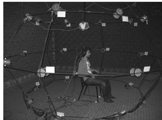
Figure 2: Construction of loudspeakers for listening test with participant sitting in chair with headrest.
